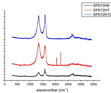
**Figure 3:** a) and b) XRD patterns, c) and d) Raman spectra of FK oxidized during 24h and 72h and reduced at different temperatures
