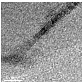
**Figure 4:** TEM of FK oxidized during 24h and reduced at temperature of 700°C
